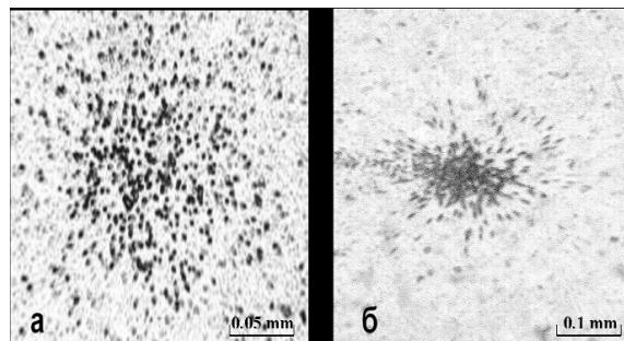
**Fig. 2.** Distribution of tracks on lysisan detector, an agglomeration: a) with high density; b) «star» form
