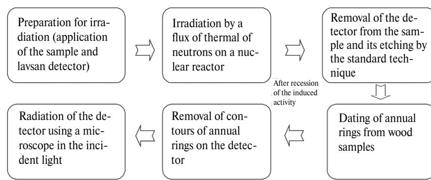
**Fig. 1.** The scheme of works at radiography of wood samples
