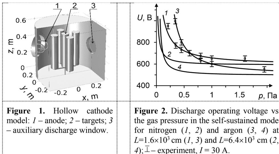
From relation (2) and Figure 2 it is seen that decreasing the effective length of the hollow cathode  $L = 4V/S_a$  (increasing the anode area  $S_a$  or decreasing the cathode volume due to targets,  $V_c - V_d$ ) increases the discharge voltage. This owes to capture of fast electrons by the anode, and the self-sustained discharge current is kept at the specified level due to the emission current (the coefficient  $\gamma$ ), i.e., due to the voltage in the cathode layer.
