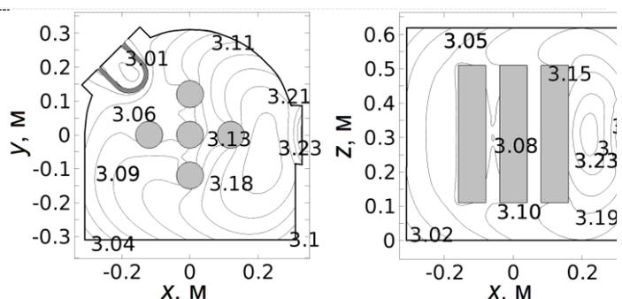
**Figure 6.** Plasma density distribution for nitrogen ( $\text{cm}^{-3} \times 10^{11}$ ) in the lateral and longitudinal sections of the hollow cathode with targets; non-self-sustained mode.
