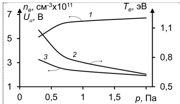
**Figure 3.** Calculated pressure dependences of the argon plasma in the self-sustained mode: 1 – plasma density; 2 – plasma temperature; 3 – plasma potential;  $S_a = 220 \text{ cm}^2$ .
