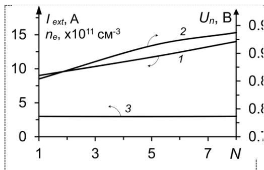
**Figure 5.** External injection current (1), plasma density (3), and plasma potential (2) vs the number of targets; nitrogen.
