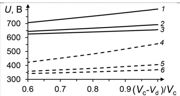
**Figure 4.** Discharge voltage in argon vs the relative volume in the self-sustained (solid lines) and non-self-sustained (dashed lines) modes at different pressures  $p$ : 0.35 (1, 4), 0.65 (2, 5), and 1 Pa (3, 6);  $\delta = 0.11$ .
