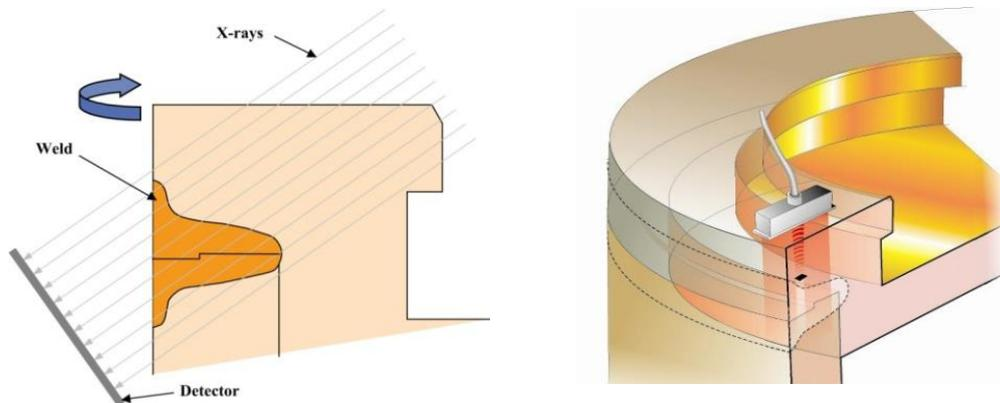
**Figure 2.** Radiography (left) and ultrasonic inspection (right) of friction welded joint.
