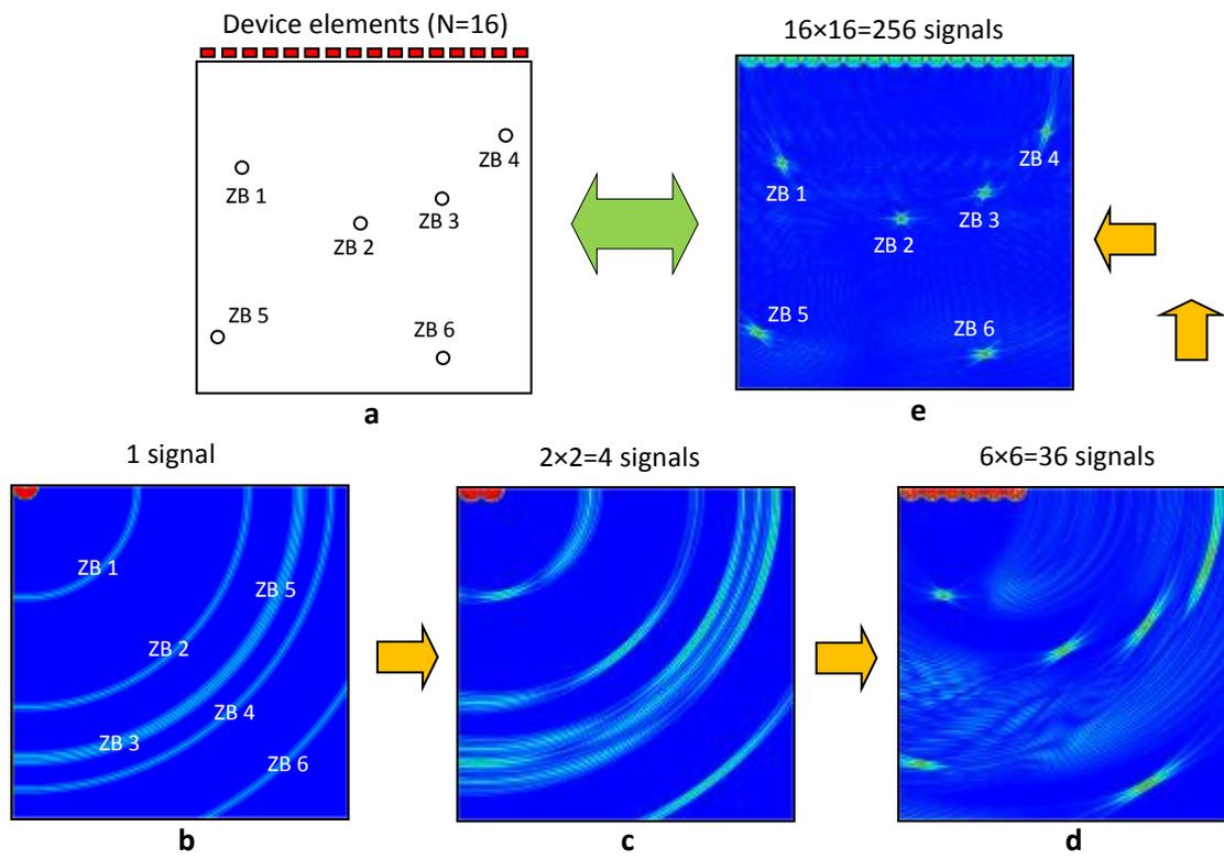
**Figure 5.** Example of image reconstruction for Sector-scan for 16 element transducer. Times of propagation of waves reflected by six side-drilled holes form the image according to DFA technique.
