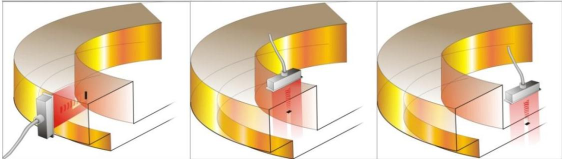
**Figure 1.** Ultrasonic inspection of cask lid.
