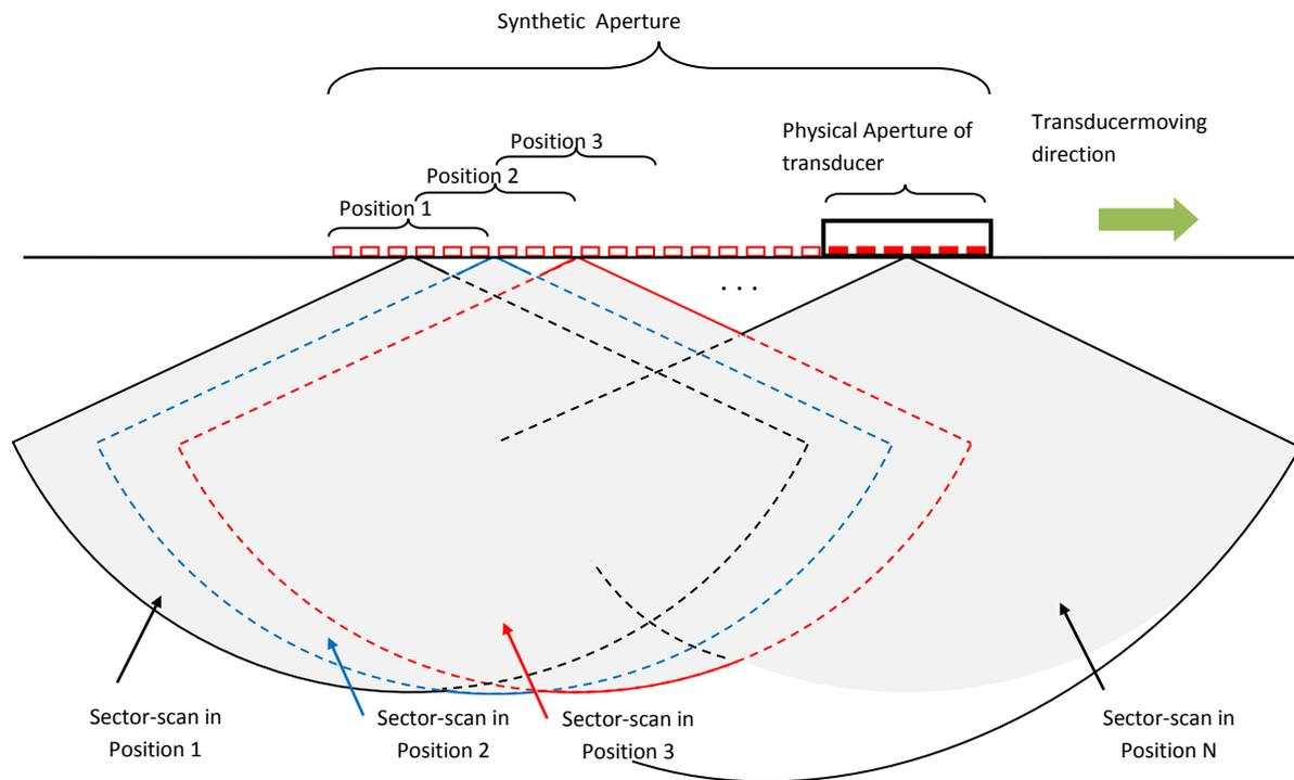
**Figure 6.** Construction of synthetic aperture.
