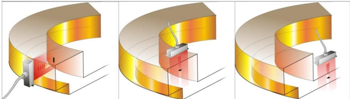
**Figure 1.** Ultrasonic inspection of cask lid.
