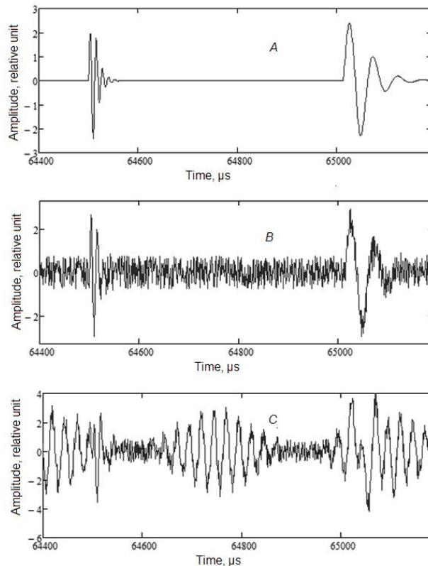
**Figure 3.** Informative electromagnetic signals of 20 kHz and 80 kHz (a); the same signals with white noise (b) white noise and sinusoidal electromagnetic interference (c).
