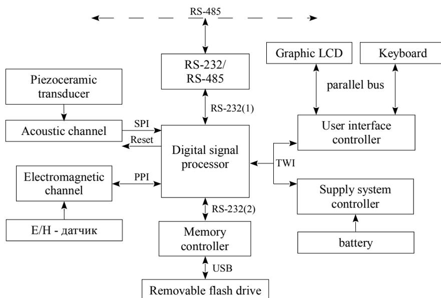
**Figure 1.** Block diagram of the recorder.
