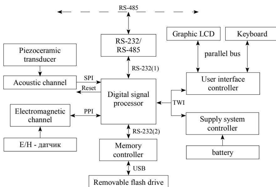
Figure 1. Block diagram of the recorder.
