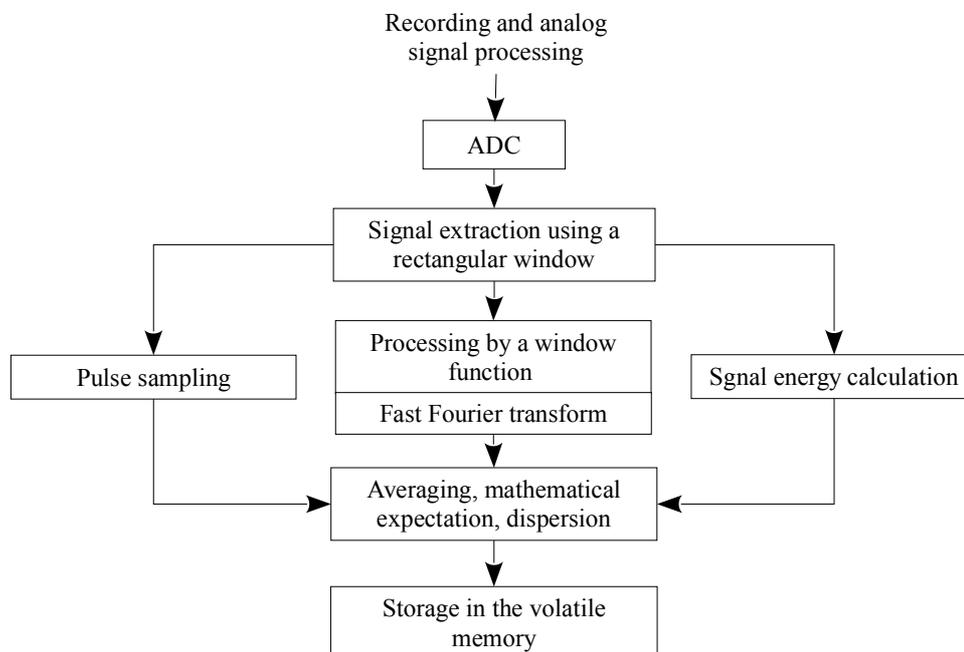
**Figure 2.** Algorithm for the mathematical block of the recorder.
