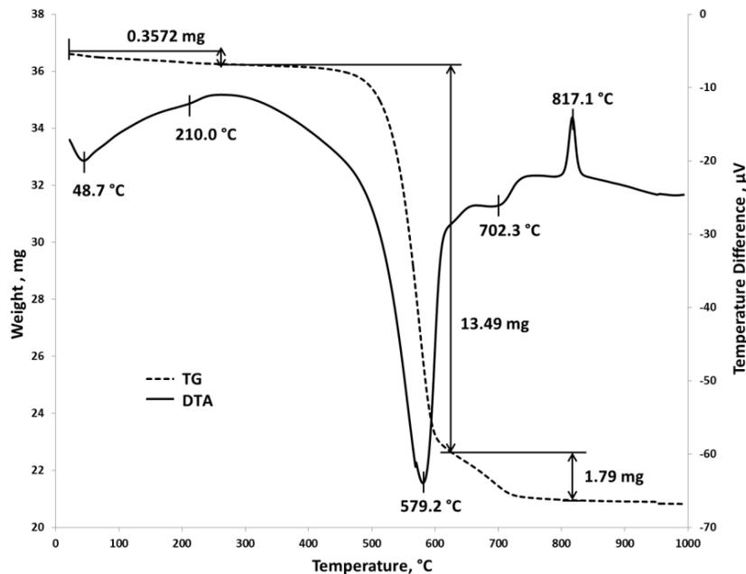
Fig. 2 Thermogram of amorphous magnesite
