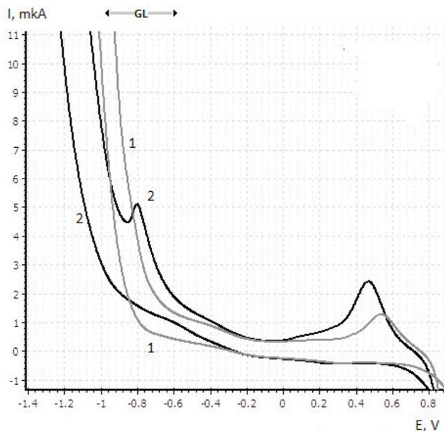
Fig.1. Cyclic voltammogram of the phosphate borate buffer with pH 9.18 in the absence (1) and in the presence of glutamate ( $4.5 \cdot 10^{-3}$  M) (2) on the CCEMG measured in the range from +0.8 to -1.4 V. The number of cycles was 3. The scan rate was  $50 \text{ mV} \cdot \text{s}^{-1}$
