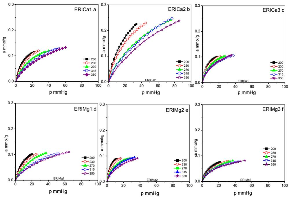
Fig. 2. Adsorption isotherms of CO<sub>2</sub> on ERICa and ERIMg zeolites.
