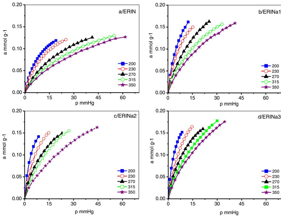
Fig. 1. Adsorption isotherms of CO<sub>2</sub> on ERIN and ERINa zeolites.
