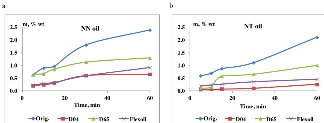
Fig. 1. (a) Time variation of oil sludge amount upon introduction of additives into NN and (b) (NT) oils
