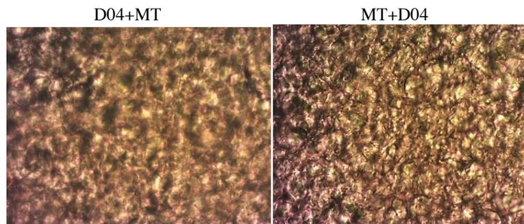
Fig.5. Photomicrographs of oil sludge extracted from oil 30 minutes after treatment
