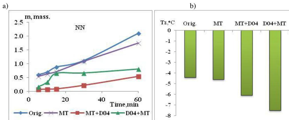
Fig. 4. (a) Time variation of oil sludge amount; (b) oil pour point after magnetic and physicochemical treatment
