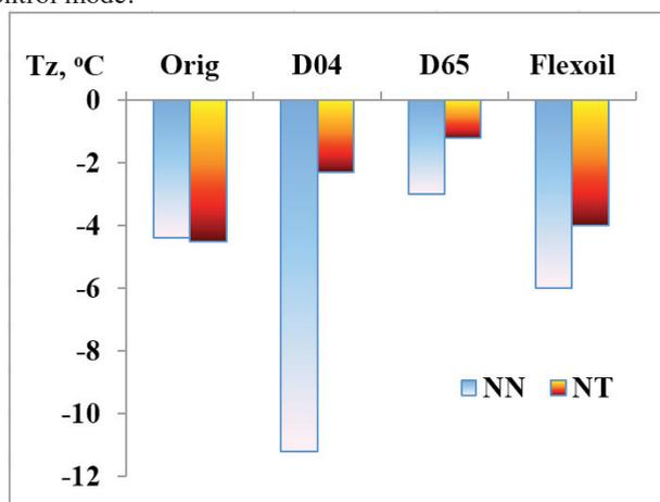
Fig. 3. Pour point of thermostatically controlled and non-thermostatically controlled oils upon introduction of additives
