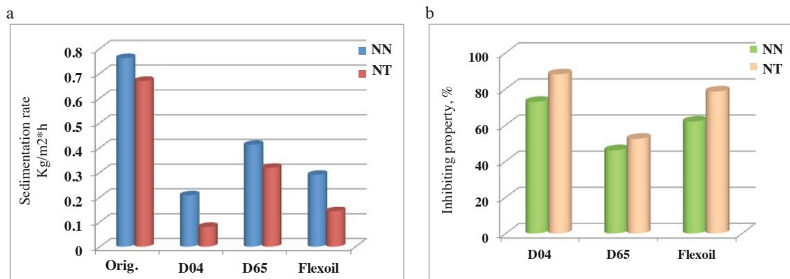
Fig. 2. (a) Sedimentation rate and (b) inhibiting property of additives for thermostatically controlled and non-thermostatically controlled oils
