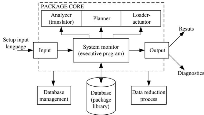
Fig. 1. Applied software packages generic architecture.
