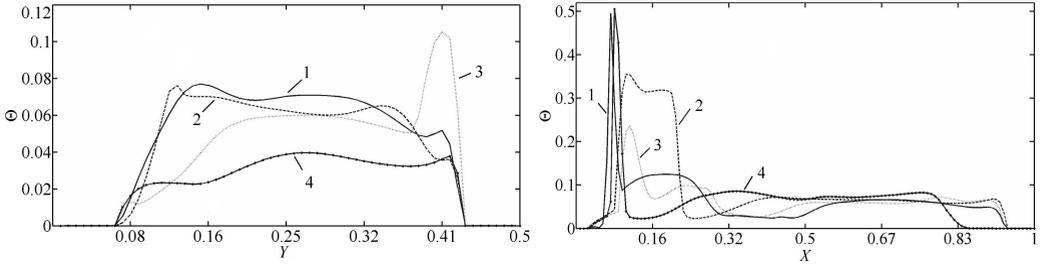
**Figure 3.** Temperature profile at sections  $X = 0.5$  (a) and  $Y = 0.5$  (b) at different  $\tau$ : 1 -  $\tau = 20000$ , 2 -  $\tau = 60000$ , 3 -  $\tau = 90000$ , 4 -  $\tau = 120000$
