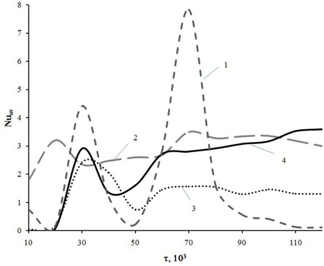
**Figure 4.** Dependence of the average Nusselt number on the time  $\tau$  at interfaces: 1 -  $X = L_1$ ; 2 -  $Y = H_{UP}$ ; 3 -  $Y = H_{LB}$ ; 4 -  $X = L_R$ .
