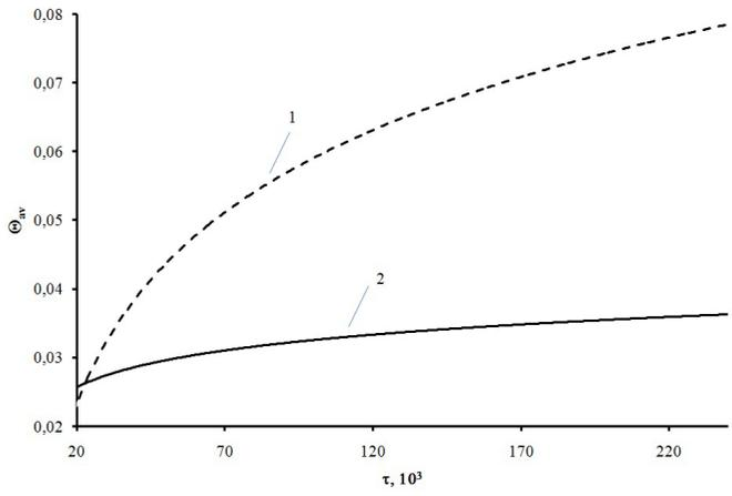
**Figure 5.** Values of the average temperature region of solutions (excluding the window aperture - 1, subject to the window aperture - 2).
