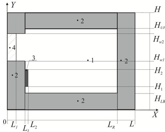
**Figure 1.** Area solution to the problem: 1 - air; 2 - enclosing structures; 3 - heat source; 4 - the window;  $L$  - size of the area in the direction  $X$ ;  $H$  - size of the solutions in the direction of  $Y$ ; Indexes:  $L, R, LB, UP$  - respectively left, right, upper and lower boundaries between media.caption.
