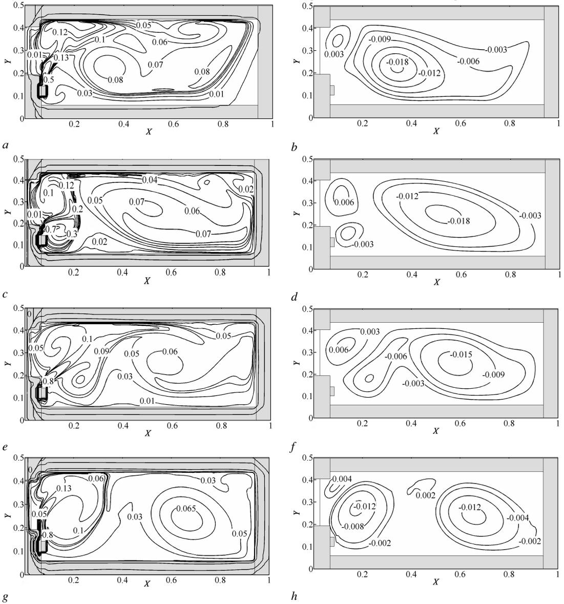
**Figure 2.** Area Temperature fields (a, c, e, g) and the contours of stream function (b, d, f, h) at different timer:  $\tau = 20000$  (a, b),  $\tau = 60000$  (c, d),  $\tau = 90000$  (e, f),  $\tau = 120000$  (g, h).
