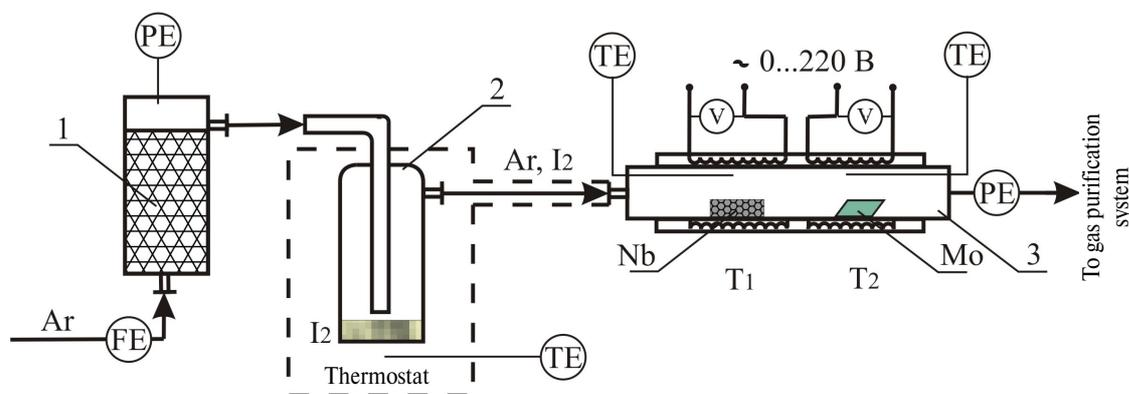
**Fig. 1.** Diagram of the laboratory device for covering niobium coating on molybdenum by gas-transport technique: 1) column of argon refining from water and oxygen vapors; 2) iodine evaporator; 3) reactor of gas-transport covering of niobium coating
