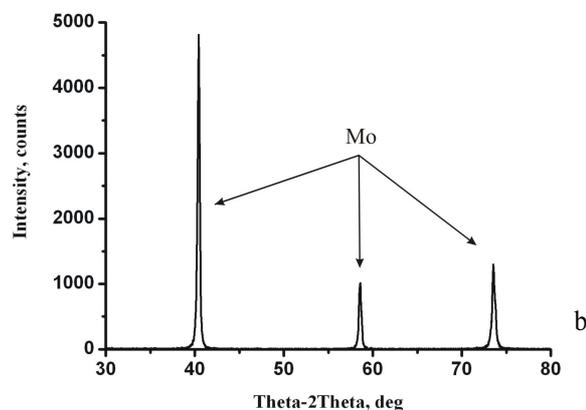
**Fig. 3.** The diffraction pattern of molybdenum plate of: a) inner and b) outer surface
