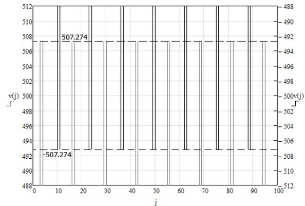
Figure 3. Positive and negative peaks of half-waves with a frequency of  $f = 1 / 13$  kHz
