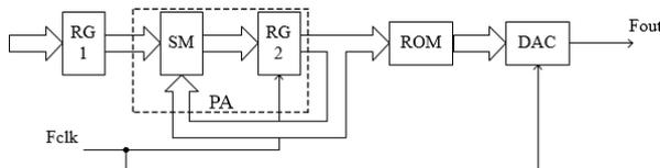
Figure.1. Function diagram of DDS generator
