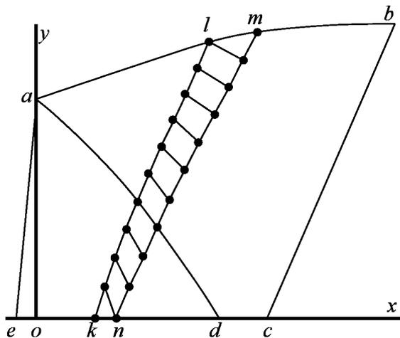
**Fig. 1.** Scheme of nozzle.  $oa$  – minimum section;  $ab$  – nozzle with angular point;  $ad$  – characteristic of  $C^+$ , belonging to beam of rarefaction wave;  $ae$  – initial characteristic of  $C^-$ ;  $kl$  – characteristic of  $C^+$ ;  $nm$  – characteristic of  $C^-$ ;  $cb$  – final characteristic of  $C^+$
