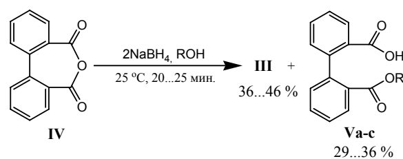
Fig. 2. Diagram of reduction of anhydride of diphenic acid \text{NaBH}_4
