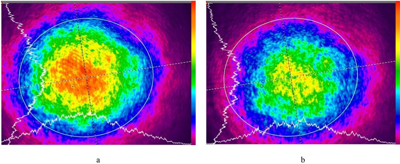
Figure 2. The distribution of the radiation intensity of the main beam (a) and beam converted into the second harmonic (b) in the first regime.
