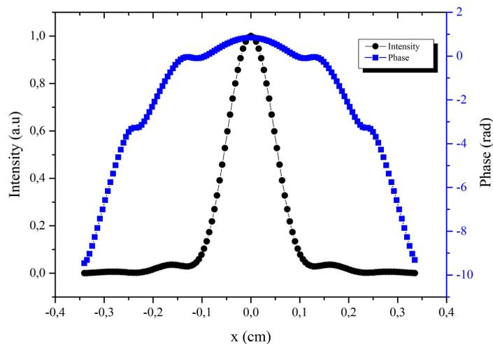
Figure 7. The intensity profile (●) and phase (■) laser beam calculated in the program FRESNEL.
