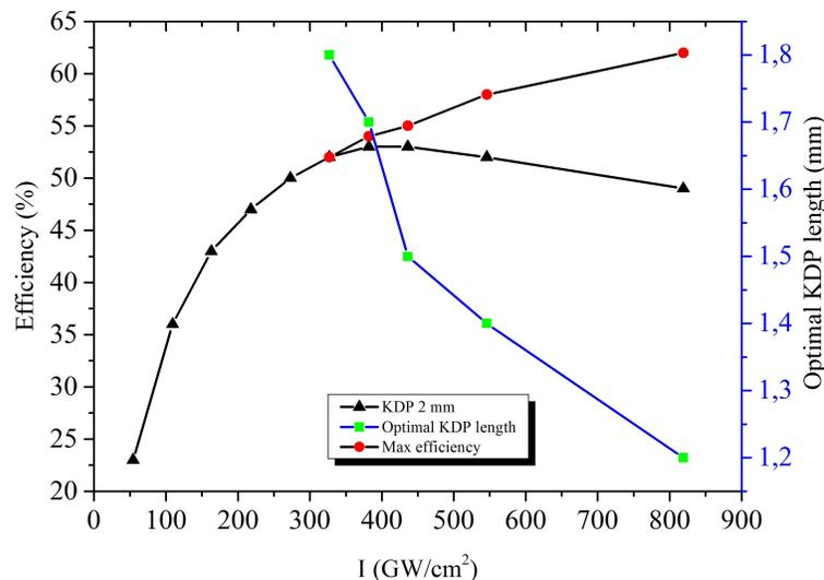
Figure 5. Theoretical dependence of the energy efficiency of SHG in KDP crystal 2 mm thick on the intensity of the first harmonic of the pulse at the entrance to the crystal ( $\blacktriangle$ ). The calculated optimum crystal thickness ( $\blacksquare$ ), necessary for high performance SHG ( $\bullet$ ).
