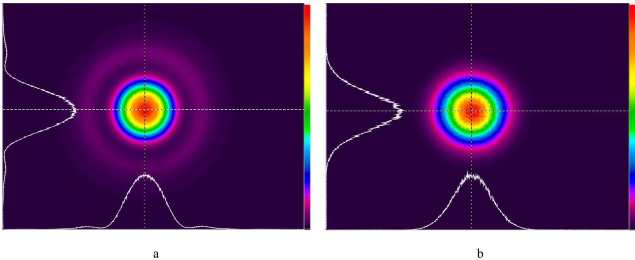
Figure 6. The distribution of the radiation intensity of the main beam (a) and beam converted into the second harmonic (b) in model experiment with beam diameter of 2 mm.
