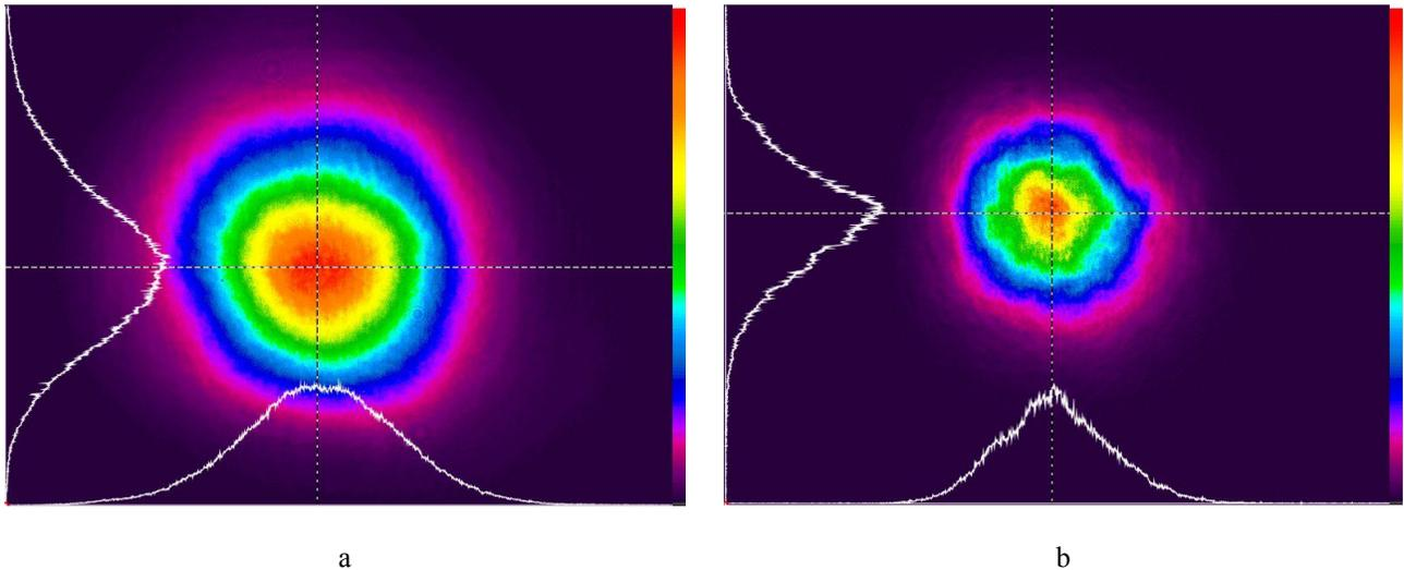
Figure 3. The distribution of the radiation intensity of the main beam (a) and beam converted into the second harmonic (b) in the second regime.
