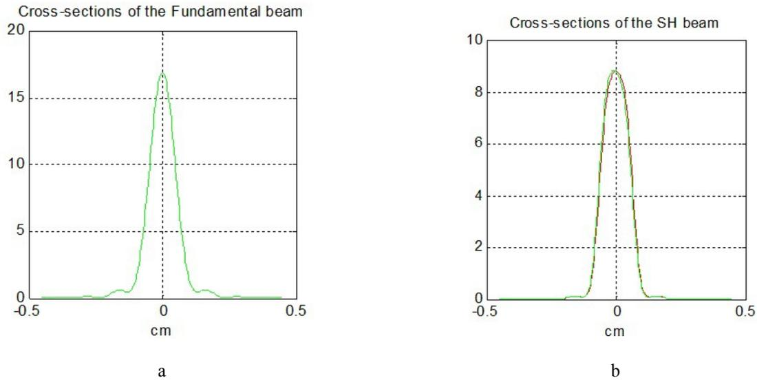
Figure 8. The cross section of the first (a) order harmonic, cross section of the infrared radiation, passing through the KDP (red), and cross section of the second harmonic (green) (b).
