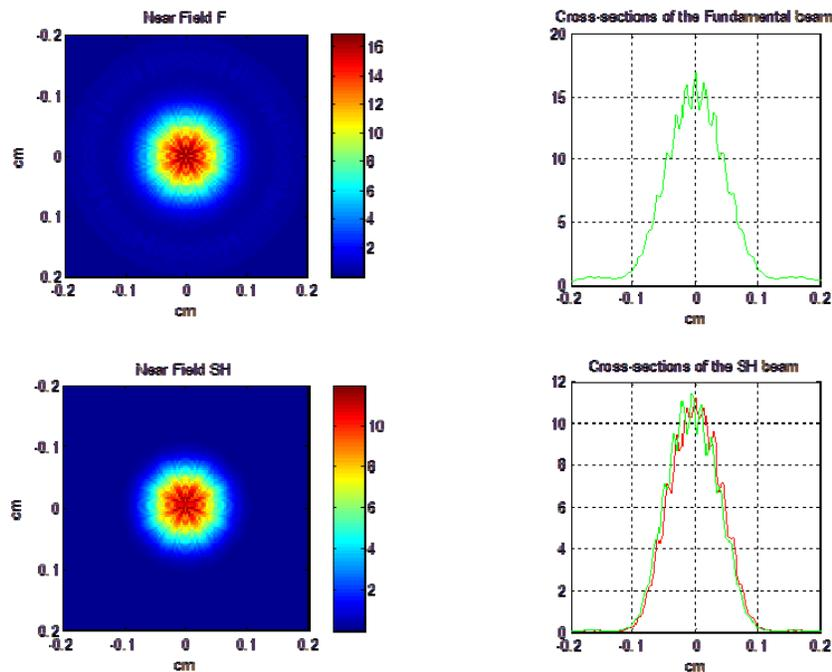
Figure 9. The intensity distribution of the initial of infrared radiation (top), infrared radiation, passing through the KDP (bottom, red) and radiation, converted to KDP (bottom, green).
