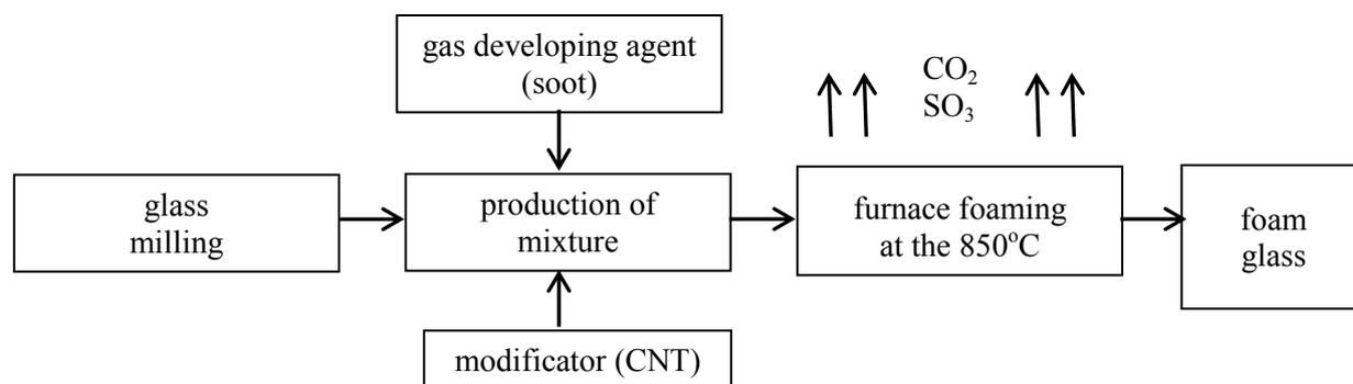
**Figure 1.** Technological scheme of foam glass producing
