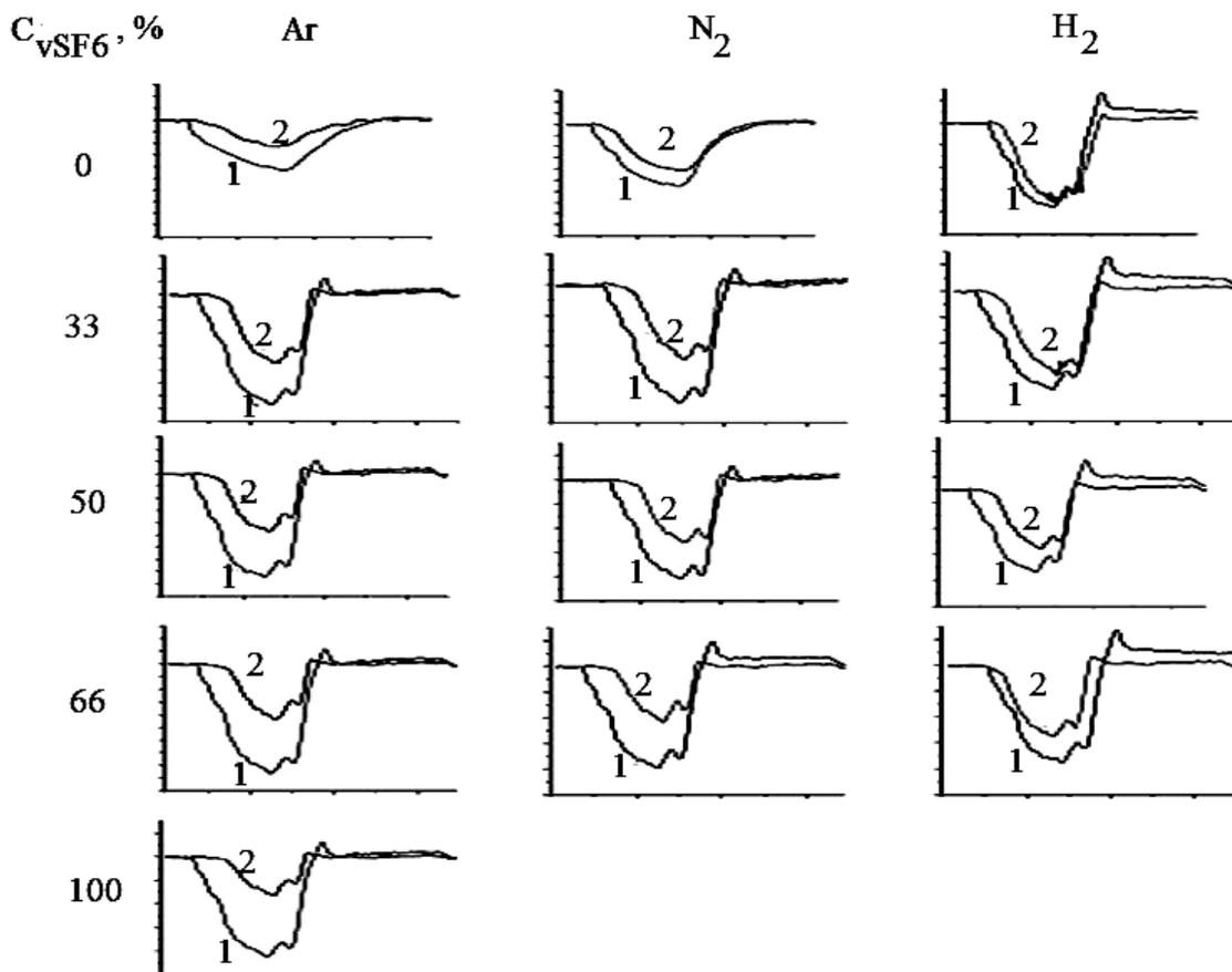
**Figure 2.** The oscillograms of the total reverse current closed on the walls of the drift tube (1) and the electron current reached the back flange of the drift tube (2).
