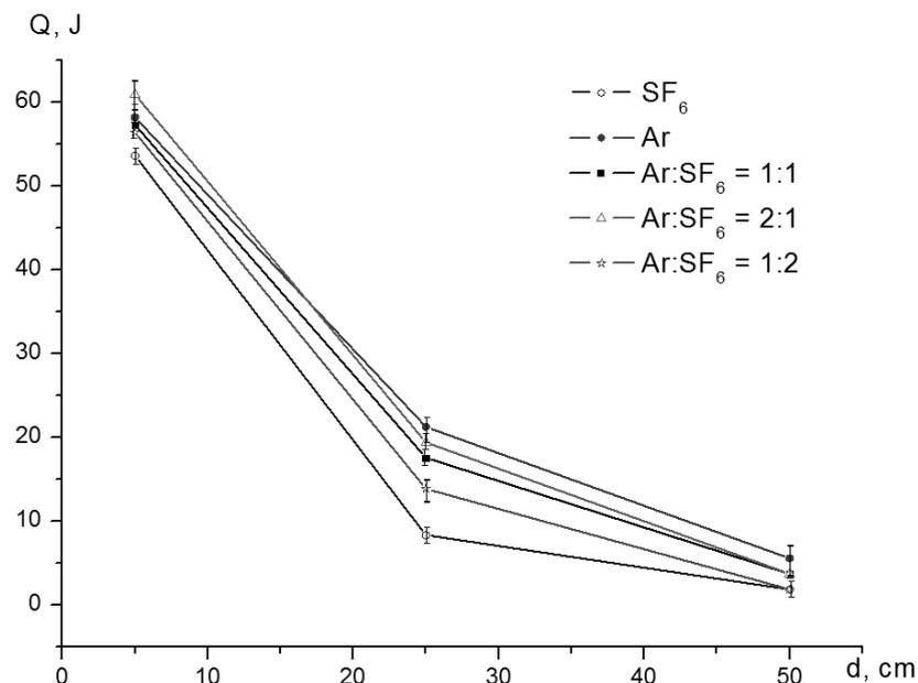
**Figure 3.** The ejected beam energy vs. the distance in the gas mixture of argon and sulfur hexafluoride, 300 Torr.
