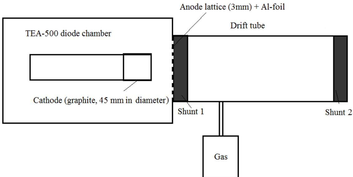
**Figure 1.** Scheme of the experimental stand to study the pulsed electron beam propagation in gases using reverse current shunts
