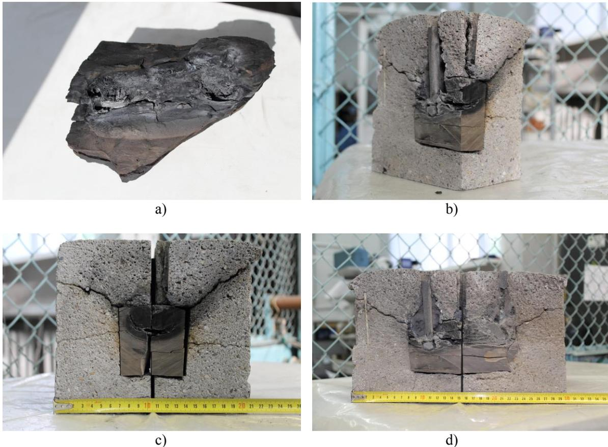
**Figure 1.** Photographs of the oil shale fragment infused in concrete after the electrophysical conversion; a) a specimen without a concrete cage, b) a lateral section, c) a longitudinal section, d) the quadrant of the sample.
