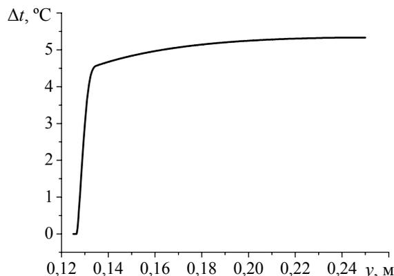
Fig. 4. Distribution of temperature difference  $\Delta t(y) = t(X_4, y, Z_k/2) - t(X_4, Y_k/2, Z_k/2)$  at the moment of time  $\tau=170$  h
