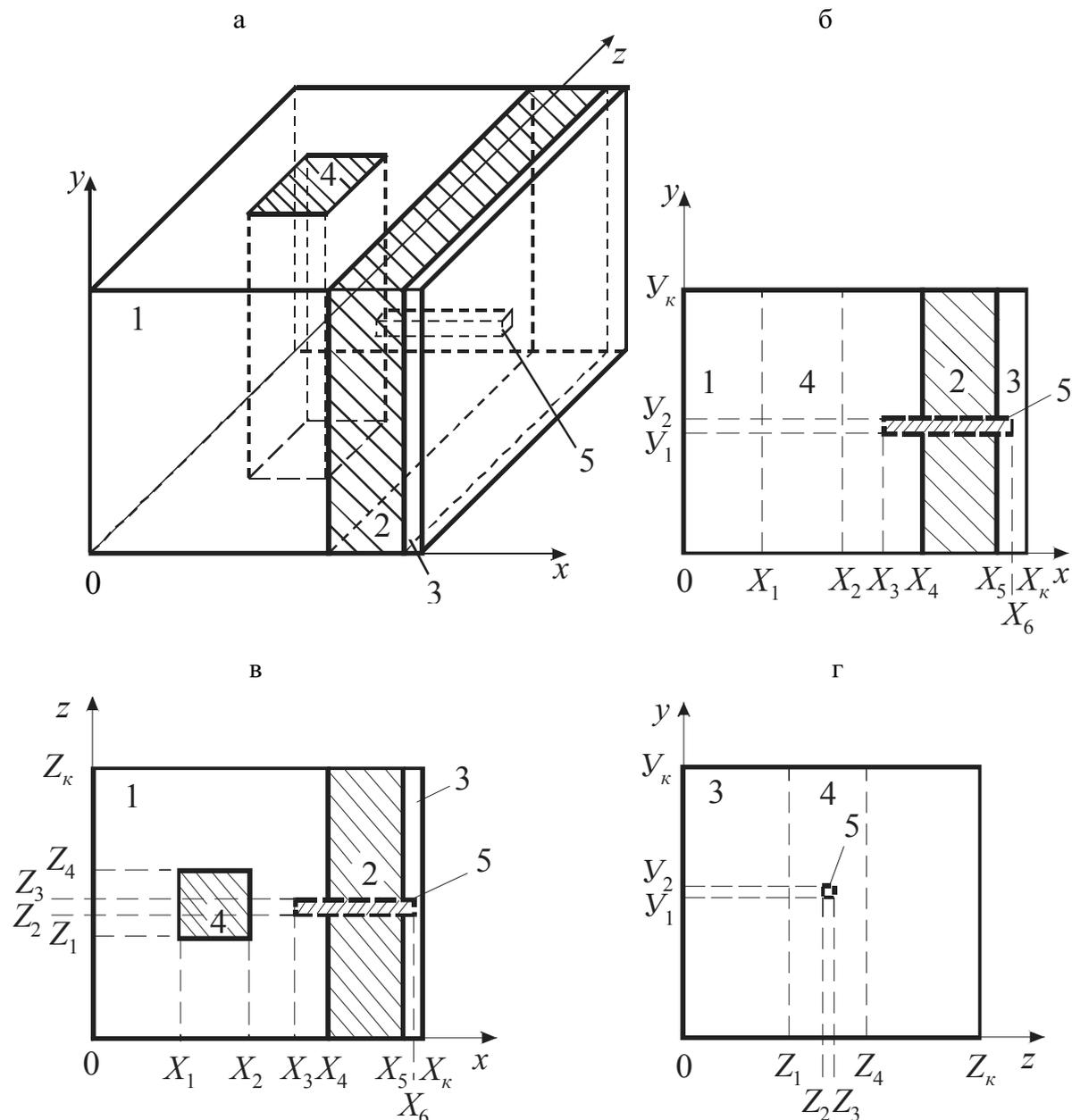
**Fig. 1.** Scheme of heterogeneous fragment of claydite-concrete wall: 1) claydite-concrete; 2) heat-insulator of face warmth-keeping system; 3) sheathing; 4) interior warmth-keeping material; 5) connector. a) general view of the fragment; b-c) side view of the fragment; d) view from above
