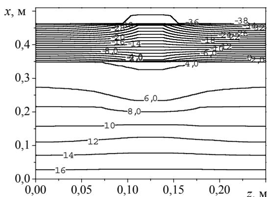
Fig. 2. Isotherms in cross-section of the fragment  $y=Y_k/2=0,125$  m, crossing the axis of connector at  $\tau=170$  h.  $t$ , °C
