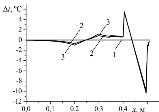
Fig. 3. Temperature difference  $\Delta t=t(x, Y_k/2, Z_k) - t(x, Y_k/2, Z_k/2)$  in thickness of the fragment with heating put in at different moments of time  $\tau$ : 1) 0; 2) 2,5; 3) 170 h
