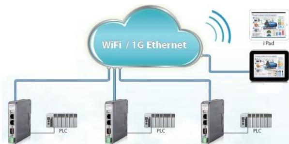
**Picture 2.** A cloud based HMI architecture
