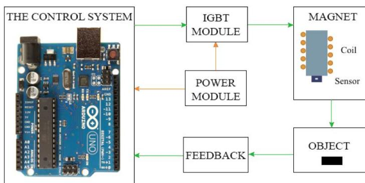
Figure 2. Schematic diagram of the system
