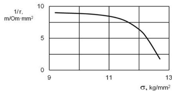
**Figure 4.** Influence of cyclic stress amplitude upon electric conductivity change
