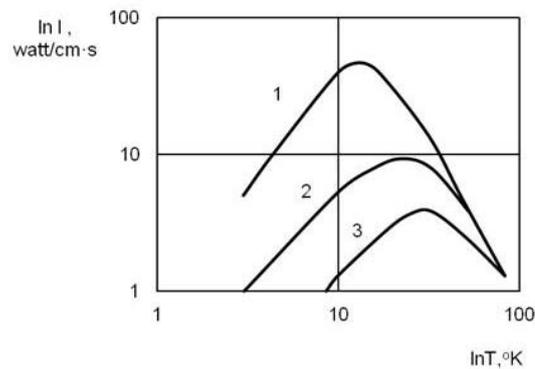
**Figure 3.** Dependence of temperature conductivity of LiF crystal upon absolute temperature under various degree of deformation: 1 – after keeping during 2 hours under 830° C ( $\rho' = 3 \cdot 10^4 \text{ cm}^{-2}$ ), 2 – after deformation of 2,4% under room temperature, ( $\rho' = 1,8 \cdot 10^7 \text{ cm}^{-2}$ ), 3 – after deformation of 4% under 180° C ( $\rho' = 4,6 \cdot 10^7 \text{ cm}^{-2}$ )
