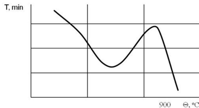
**Figure 2.** The curve of the temperature-tool life
