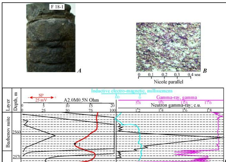
**Figure 6.** Structure (A), petrographic composition (B) and geophysical characteristics (C) of Bazhenov suite bituminous hydromica argillites with pyrite: A – Well 18 Fobosskaya, depth=2598.0 m; B – Well 18 Nizhe-Tabaganskaya, depth=2564.0 m; C – Well 18 Fobosskaya; depth=2598.0 m.
