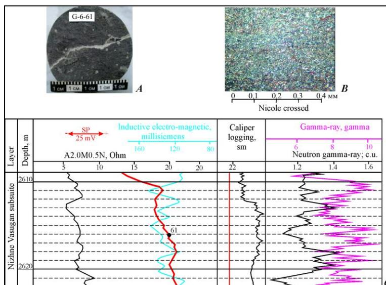
**Figure 4.** Structure (A), petrographic composition (B) and geophysical characteristics (C) of Nizhne-Vasugan subsuite hydromica clay rocks: A, B, C – Gerasimovskaya-6; depth= 2616.0 m.
