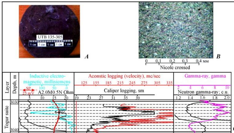
**Figure 5.** Structure (A), petrographic composition (B) and geophysical characteristics (C) of Togur subsuite bituminous hydromica argillite with pyrites and fine-grained quartz impurities: A, B, C – Well 135 South-Tabaganskaya; depth=3033.5 m.
