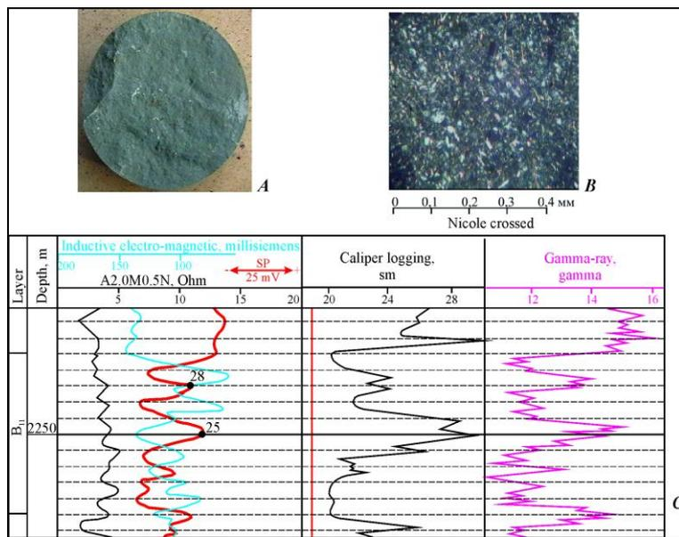
**Figure 3.** Structure (A), petrographic composition (B) and geophysical characteristics (C) of chlorite-hydromica clays of marine genesis: A, B, C – Well 213 Sobolinaya; depth= 2225.0 m
