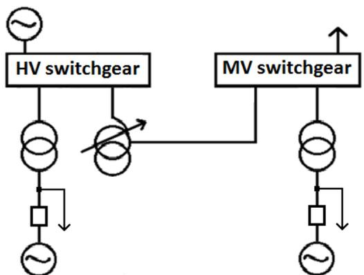
Figure 2. Power plant simplified block diagram with connection power autotransformer.
