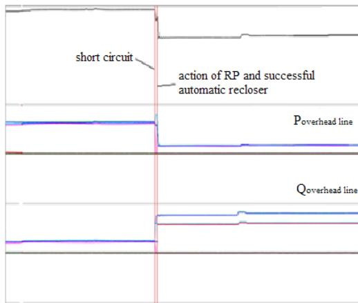
**Figure 6.** Real time data oscilloscope of changing loads on time feeder short-circuit, CSR and banks of capacitors switching-off.
