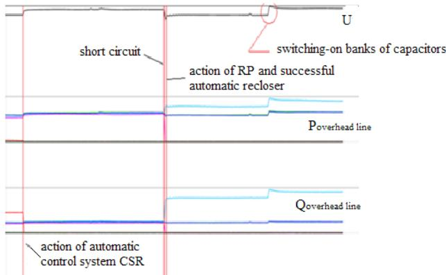
**Figure 5.** Real time data oscilloscope of changing loads on time feeder short-circuit, CSR and banks of capacitors switching-on.
