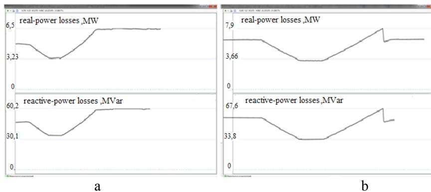
**Figure 7.** Real time data oscilloscope of total power losses in Elgaugol a - CSR and banks of capacitors switching-on, b - CSR and banks of capacitors switching-off.
