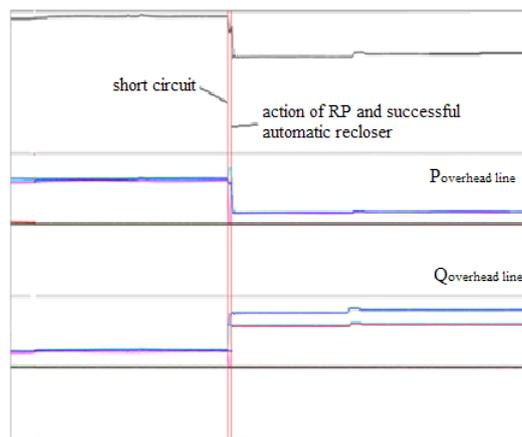
**Figure 6.** Real time data oscillogram of changing loads on time feeder short-circuit, CSR and banks of capacitors switching-off.
