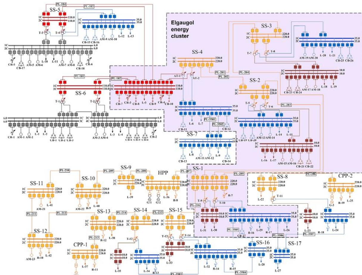
**Figure 2.** Simulated power system: SS – substation, CPP – co-generation power plant, HPP – hydro power plant, PL – power line, CB – capacitors bank, CR – controlled shunt reactor, R – switched reactor, L – load, AM – asynchronous motor, G – generator, (A)T – (auto) transformer.
