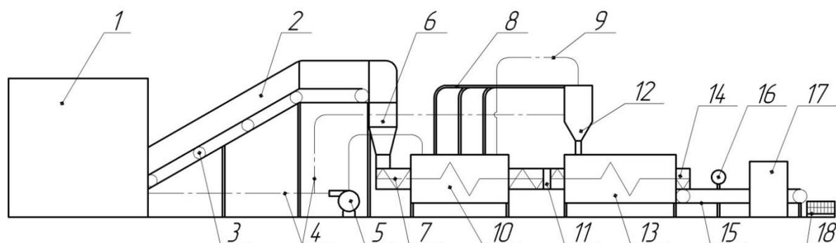
**Figure 1.** Layout diagram of the process line at small-tonnage solid composite fuel production: 1 – storeroom, 2 – dry of raw, 3 – conveyer, 4 – conduit of flue gases, 5 – exhauster, 6 – grinder, 7 – conveyer screw, 8 – conduit of volatile products, 9 – conduit of gas, 10 – combustion chamber, 11 – box-coupling, 12 – unit of binder preparation, 13 – heat-exchange unit, 14 – conveyer screw, 15 – conveyer, 16 – press roll, 17 – molder of stamping, 18 – dilly.
