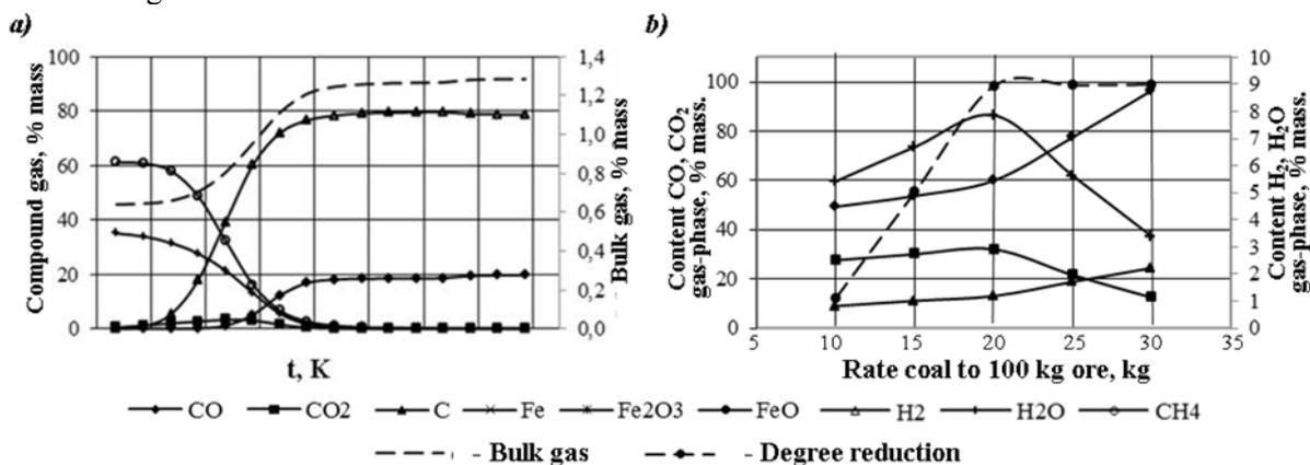
a – the dependence of the volume and composition of gas phase temperature;
