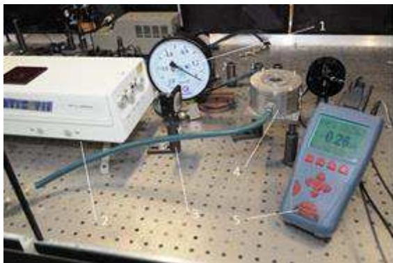
Pic.1. The general view of the experimental set. 1-monometr, 2-laser set, 3-lens, 4-box furnace, 5-power meter
