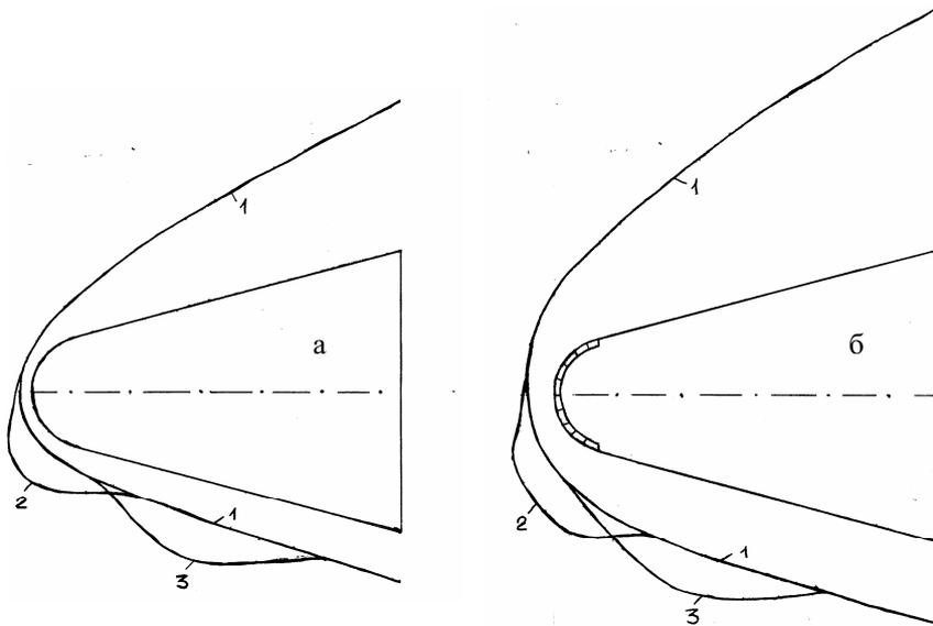
Fig. 1. Patterns of supersonic flow of body surface: 1)  $t=0$ ; 2)  $t=2,82, y_0=-y_c$ ; 3)  $t=6,84, y_0=-1,75$ : a) at blowing; b) without blowing
