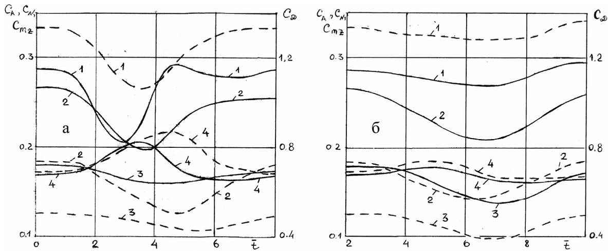
Fig. 2. Dependencies of aerodynamic properties  $C_A(1), C_N(2), C_{mz}(3), C_o(4)$ ; — — without blowing; - - - with blowing: a)  $y_0=-y_c$ ; б)  $y_0=-1,75$
