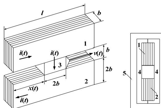
Fig. 1. Railgun schematic circuit: 1) and 2) rails consisting of isolated plates; 3) accelerated body; 4) insulation; 5) fasteners;  $v(t)$  is the body velocity;  $x(t)$  is the distance covered by the body in railgun;  $i(t)$  is the electric current;  $l$  and  $b$  are the length and width of rails
