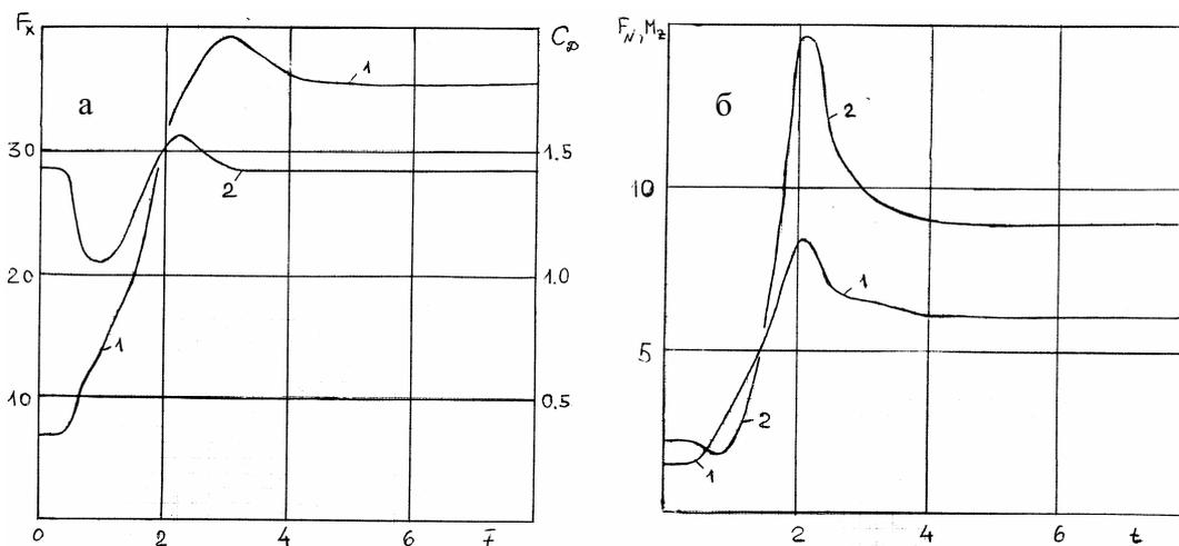
Fig. 4. Dependencies of aerodynamic properties on time: a) 1 -  $F_A$ ; 2 -  $C_D$ ; b) 1 -  $F_N$ ; 2 -  $M_z$
