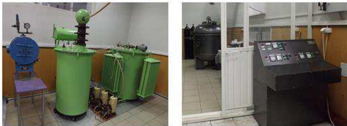
Fig. 2. – Small chamber, power supply with regulators and commutation system (left photo), control panel and big chamber (right photo)
