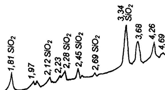
**Fig. 7.** Roentgen diffractograms of coal fraction of 1600...2280 kg/m<sup>3</sup> density
