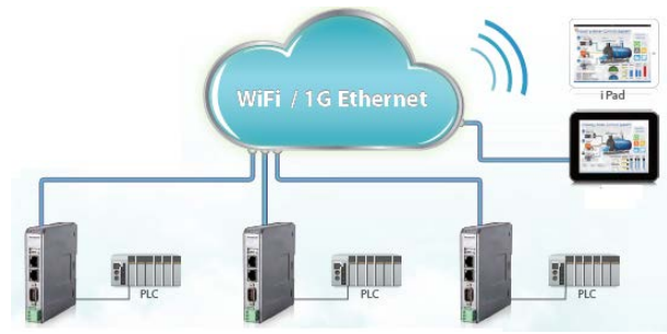
Figure 3. cloud based HMI architecture
