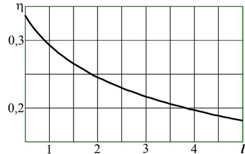
Fig. 4. Dependence of transformation efficiency on railgun length (in meters) at  $V_0=0,1$  km/sec;  $V_m=3$  km/sec;  $m=0,1$  kg;  $\rho=3$  g/sm<sup>3</sup>
