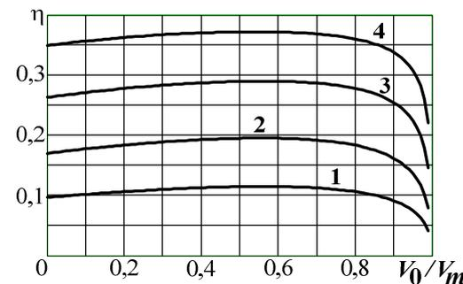
Fig. 6. Dependence of transformation efficiency on relative initial body velocity at  $V_m=3$  km/sec;  $l=1,94$  m: 1)  $m=10^{-3}$  kg and  $\rho=1$  g/sm<sup>3</sup>, 2)  $m=10^{-2}$  kg and  $\rho=3$  g/sm<sup>3</sup>, 3)  $m=10^{-1}$  kg and  $\rho=10$  g/sm<sup>3</sup>, 4)  $m=1$  kg and  $\rho=20$  g/sm<sup>3</sup>
