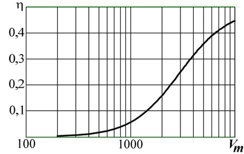
Fig. 3. Dependence of transformation efficiency on maximum velocity of accelerated body (in m/sec) at  $V_0=0,1$  km/sec;  $m=0,1$  kg;  $l=1,94$  m;  $\rho=3$  g/sm<sup>3</sup>
