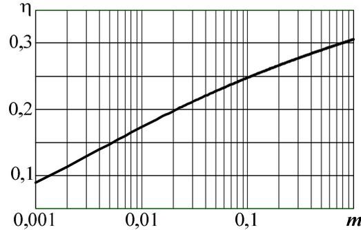
Fig. 2. Dependence of transformation efficiency on weight of accelerated body (in kg) at  $V_0=0,1$  km/sec;  $V_m=3$  km/sec;  $l=1,94$  m;  $\rho=3$  g/sm<sup>3</sup>
