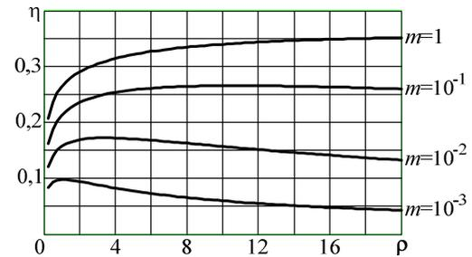
Fig. 5. Dependence of transformation efficiency on volume density of accelerated body (in g/sm<sup>3</sup>) for its different weight  $m$  (in kg) at  $V_0=0,1$  km/sec;  $V_m=3$  km/sec;  $l=1,94$  m
