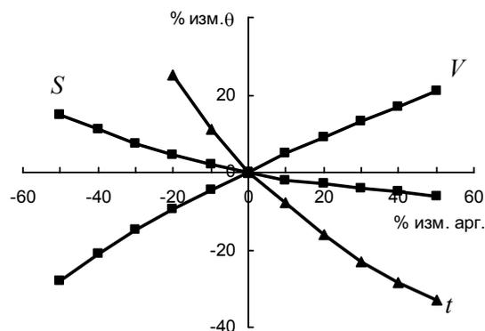
Fig. 3. Influence of cutting mode elements of on cutting temperature
