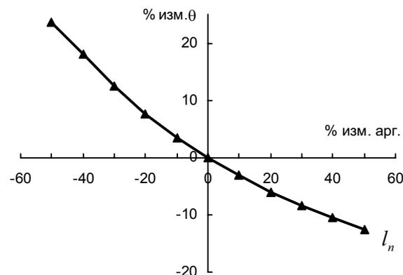
Fig. 6. Influence of contact length on a front surface of a cutter on cutting temperature
