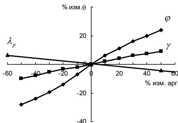
Fig. 2. Influence of coefficient of heat conductivity of a tool material ( $\lambda_p$ ), the main angle in the plan ( $\varphi$ ) and a front angle in the in main secant plane ( $\gamma$ ) on cutting temperature
