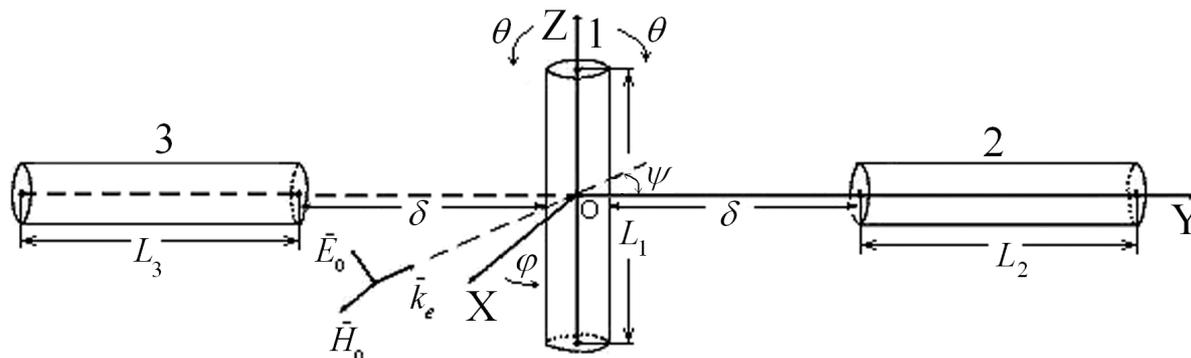
Fig. 4. Structure from mutually orthogonal conductors
