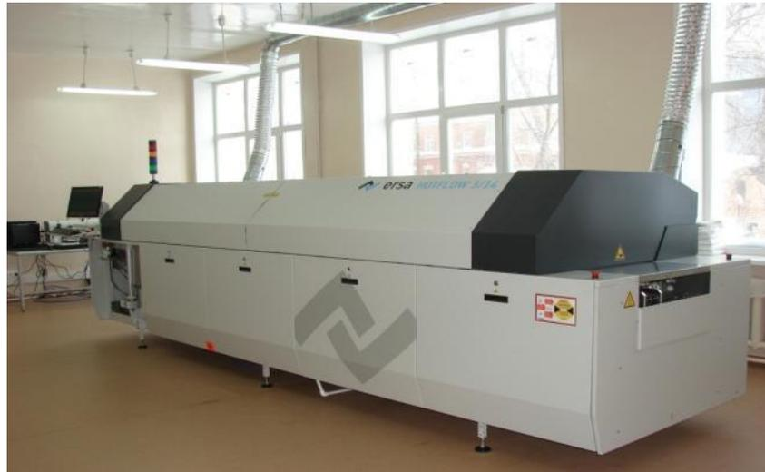
Fig.7.9 – ErsaHotflow 3/14 convection reflow furnace
