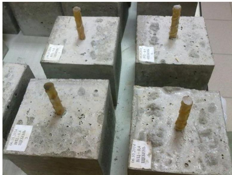
Figure 19 – Samples of concrete reinforced by GFRP bars
