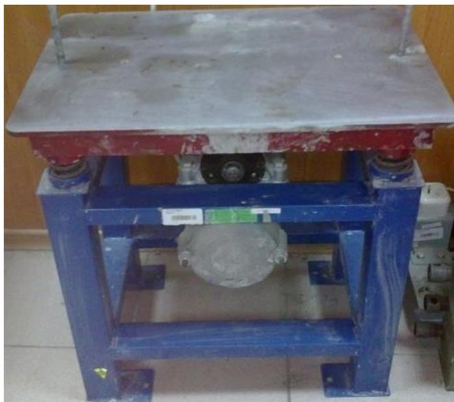
Figure 18 – Laboratory vibrating platform CMЖ-539
