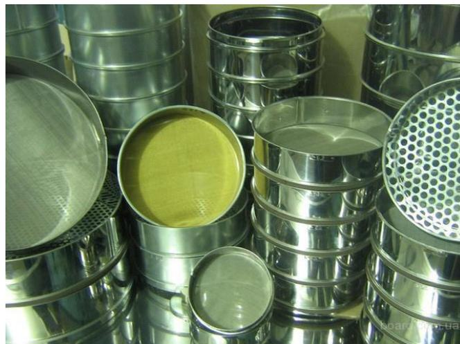
Figure 15 – The laboratory sieves
