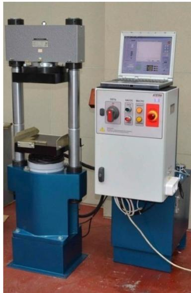
Figure 13 – The hydraulic test press III-500
