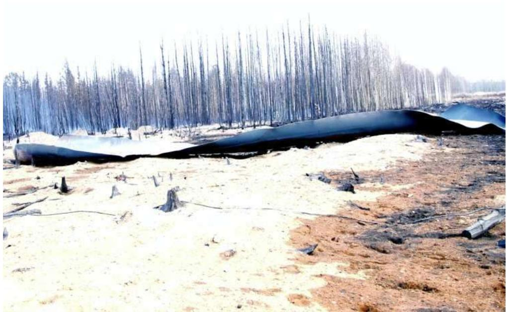
*Fig. 2. Fragments of gas pipeline destroyed by SCC*
