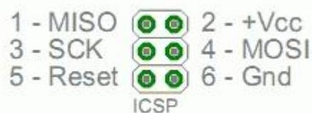
Fig. 1.2 –In-Circuit Serial Programming joint
