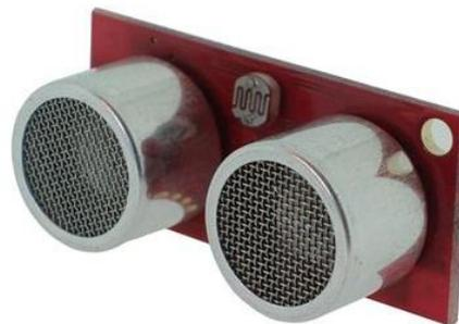
Fig. 7 Ultrasonic sensor
