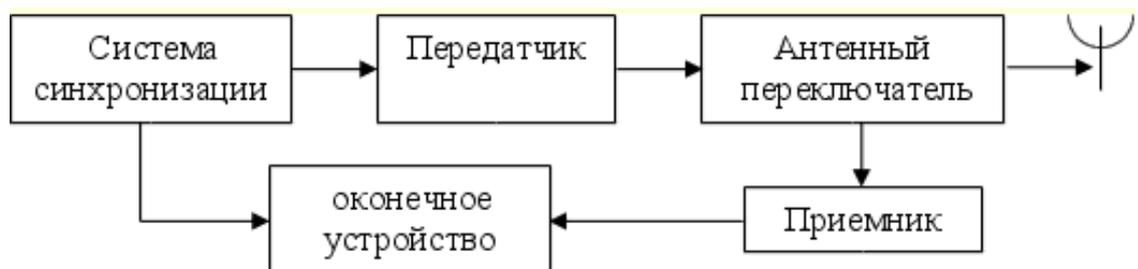
Figure 1.4 –Block diagram of the impulse method
