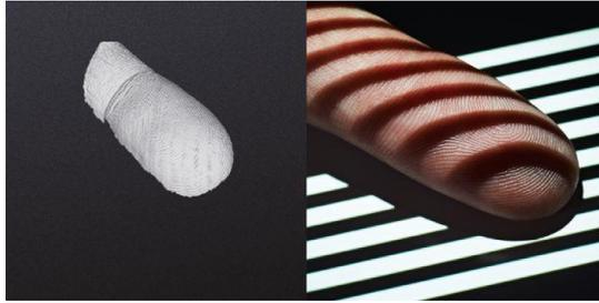
Figure A.4- The projected light pattern onto the subject
