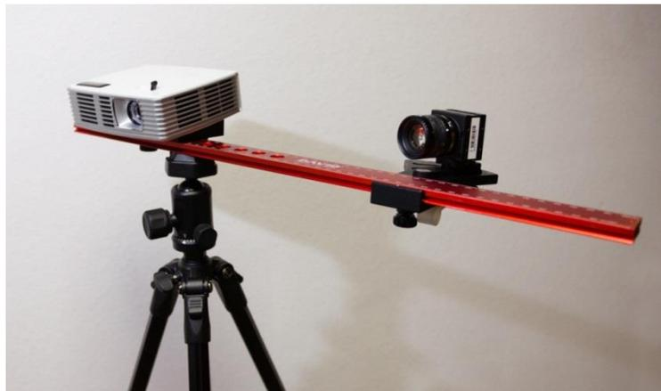
Figure A.3- physical form of the 3D scanner
