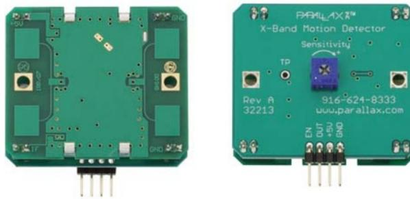
Figure 4 - Front and rear side of the X-band motion detector
