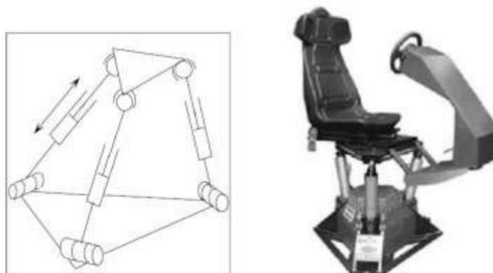
Figure 1.1.3. The manipulator with the three degrees of freedom offered by Hunt and Lee and the example of its application as an entertainment motion base.
