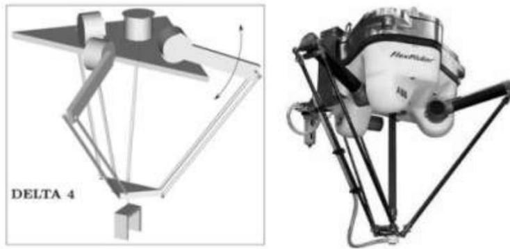
Figure 1.1.2. The Delta robot and one of its industrial implementation - the FlexPicker IRB
