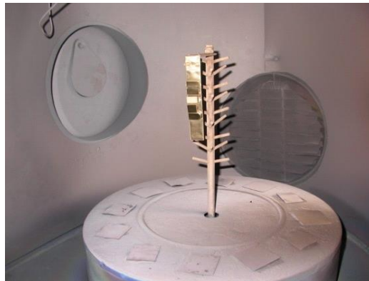
Figure 3.2.1.1 the Location of the samples in the installation
