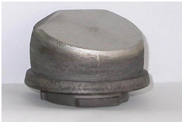
c)- composite cathode powder system Ti-Al-Si after a few cycles in a curvilinear plasma duct.;
