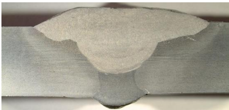
Figure 11 - The macrostructure of the weld metal: a - DC reverse polarity ; b - a rectangular alternating current of high frequency .
