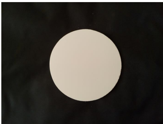
Figure 6 – Sintered target of HA that will be placed on the magnetron
