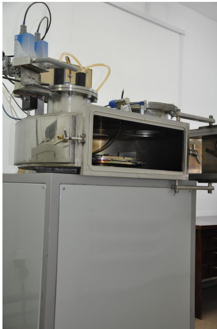
Figure 5 – Vacuum installation equipped with the source of ions, magnetron system and rotating table with a heating plate
