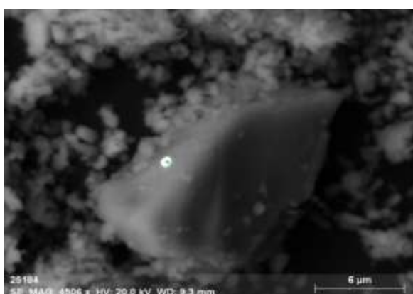
Figure 4.1.7. Micromineral phase of Pt in the hydroxyapatite aggregate in the HOAR of Norilsk residents.
