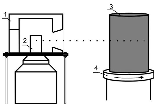
Fig. 1. Bench of radiation control of low-active SRW activity: 1) lead sheath with collimator; 2) Ge-detector; 3) standard steel container with waste; 4) electromechanical rotator
